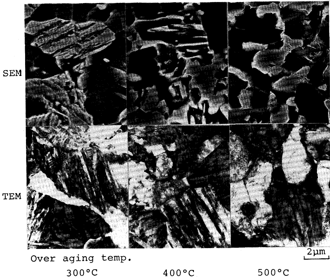
Photo. 2. SEM and TEM microstructures of direct aging (DA) type cold rolled dual phase steels (Steel 3).
