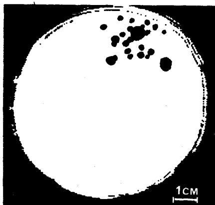
Photo. 2. Photograph obtained by UST on flash welded zone of 76 mm chain link. An arrow shows the inside of link.
