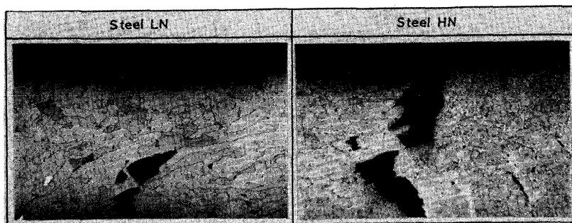
Photo. 2 Crack in edge of rolled specimen
