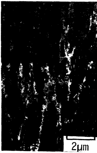
Photo. 5. Longitudinal section of the specimen cold worked 90% reduction and aged for 300 ks at 650K imaged by (201) \alpha diffraction.
