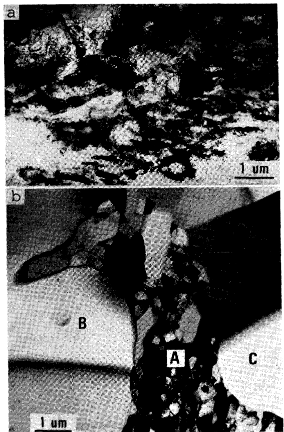
(a) Annealed for 1h at 500^\circ\text{C} . (b) Annealed for 1h at 600^\circ\text{C} . Photo. 3. Electron micrographs of cold-rolled and annealed Ti-47.5Ni-2.5Fe(at%) alloy.
