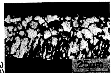
Fig.4 Optical micrograph of the longitudinal cross section of as rapidly solidified Fe-32Cr-8Ni alloy, (wheel surface velocity of 42m/s)
