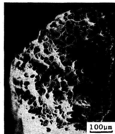
Photo. 1 Fracture Surface of SiC/Al Preform Wire Bending Test Specimen.
