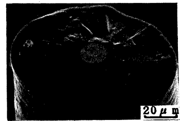
Photo.1 SEM image of cross section of boron fiber
