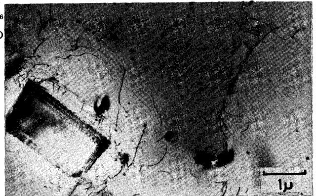
Photo. 2. 4W 1100°C, 1.2 kgf/mm 2 , 2690 hr Creep ruptured
