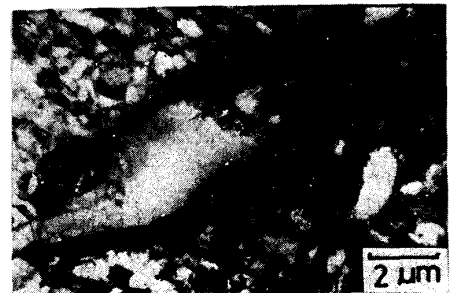
Photo. 1 TEM micrograph of 9Cr-4W-0.1C steel tempered for 1 hr at 800°C.
