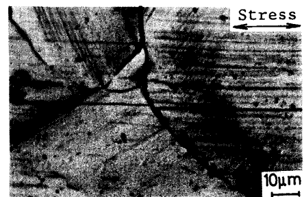
650°C, 20kgf/mm 2 , t=200h (t/tr=0.9), ε=5% Photo.1 Displacement of scratch by grain boundary sliding.
