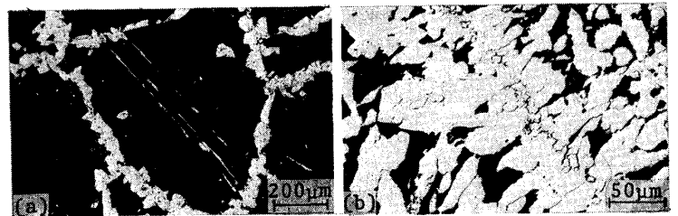
Photo.2 Optical micrographs showing the effect of the degree of deformation on the morphology of \alpha nucleated on the annealing twin boundaries in large austenite grains. (a) 10% deformed, (b) 50% deformed.
