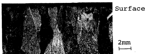
Photo 1 Macro pattern of longitudinal section showing \gamma -structure
