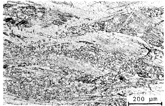
Photo. 2. Recrystallization behavior of c.p. titanium of coarse grain structure. (material T1, heating temp, 1 000°C, deformation temp, 700°C, holding time 2 s, \epsilon = 1.0 , \dot{\epsilon} = 10 \text{ s}^{-1} )
