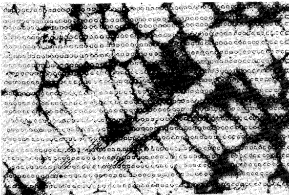
Photo. 2. Dendrite morphology of commercial steel containing 0.28wt% C quenched at 1486 °C after continuous cooling. Circles are traces of XMA. ( \times 100 )
