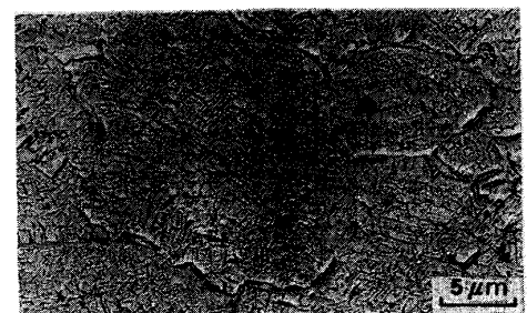
Photo.1. Electron micrograph of replica from specimen A aged at 500°C for 32h after solutioning at 650°C for 1h.
