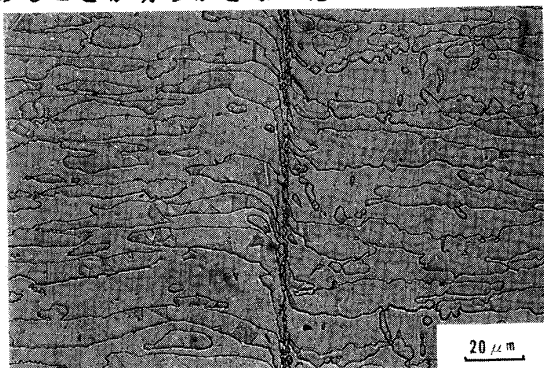
Fig. 1 Example of microstructure near bonded line
