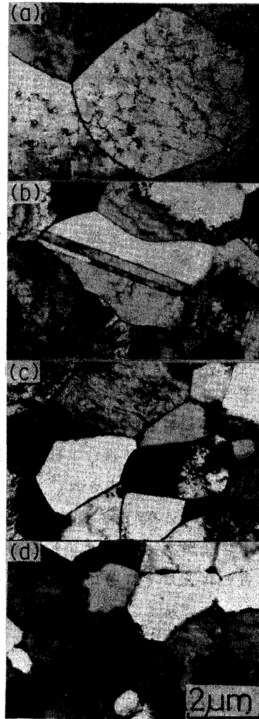
Fig.3 TEM microstructure of as rapidly solidified specimens (a) Fe-22Cr-18Ni, (b) Fe-25Cr-13.5Ni, (c) Fe-25.5Cr-13Ni, (d) Fe-30Cr-11Ni.
