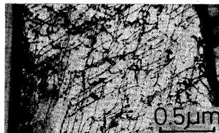
Fig.4 TEM microstructure of as rapidly solidified Fe-25.5Cr-13Ni
