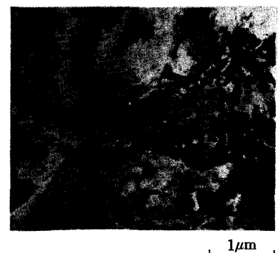
Photo.1 Thin-foil electron micrograph showing the decomposition of retained austenite in the specimen quenched with H3 and tempered at 550°C×2h.
