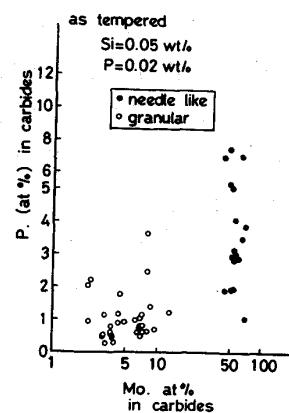
Fig. 1 Morphology and composition of carbides in 2.25Cr-1Mo steel after normalizing observed by STEM-EDX
