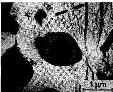
Photo.1 Typical Microstructure after 1st Heating(775 ^{\circ} C WQ)
