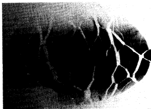
Fig. 1. Transmission Laue 211 spot of a secondary recrystallization grain grown by temperature-gradient controlled annealing.
