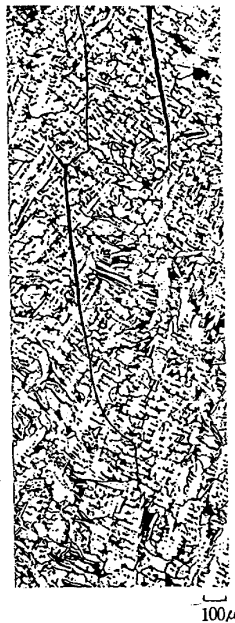
Photo 1. Micro structure of transverse crack.
