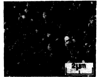
b) dust particles sampled by the tuyere probe, C% 37
