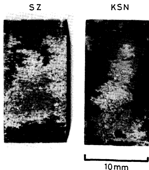
Photo. 1. Specimen appearance of the alloys SZ and KSN corroded in steam at 800°C and 40 atm for 1000 h, showing a spalling of the surface oxides.
