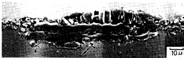
Photo. 4. Scanning electron micrograph of the cross section of nodular oxide formed on Inconel 617 corroded in steam at 800°C and 40 atm for 3 000 h.
