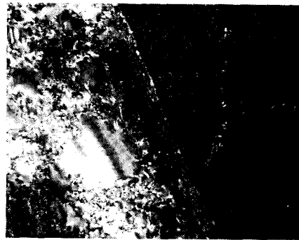
Photo. 8. Deformation structure of the aged specimen deformed at 873K.
