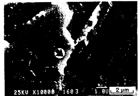
Photo.2 Bubble cavities detected by SEM in heat affected zone of elbow (20B)
