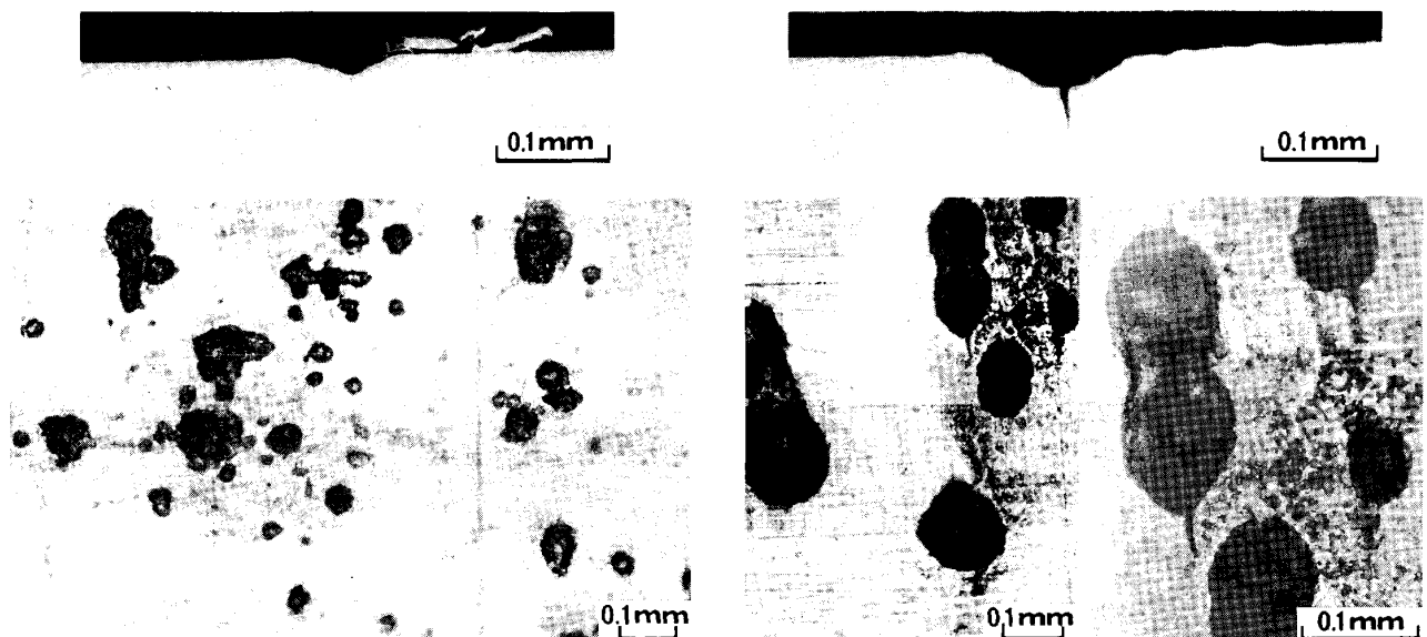
(a) Surface state of (a), N = 20 \times 10^4 (b) Surface state of (b), N = 40 \times 10^4 Fig.3 Observation of pit and crack initiation (HT60, \sigma_a = 147 \text{ MPa} , 150 rpm, N_F \approx 165 \times 10^4 )
