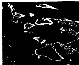
Photo 1 Martensite islands observed in the specimen with double thermal cycles(1400℃+800℃)
