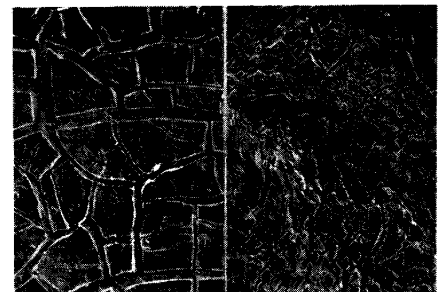
Photo. 1 Observation of surface after equi-biaxial stretching (Ex=26.5%)
