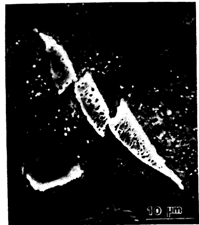
Photo. 6. SPEED Observation of cracked (Fe, Mn) 3 P after hot rolling.
