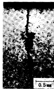
Photo. 1 Crack of carburized zone
