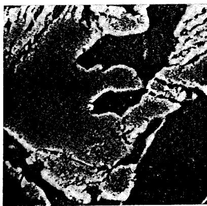
Photo. 1. Microstructure of heated to A_{C1}/A_{C3} of V added steel
