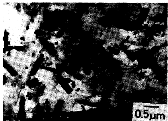
Fig. 2 Intergranular carbides observed in the unfailed tube
