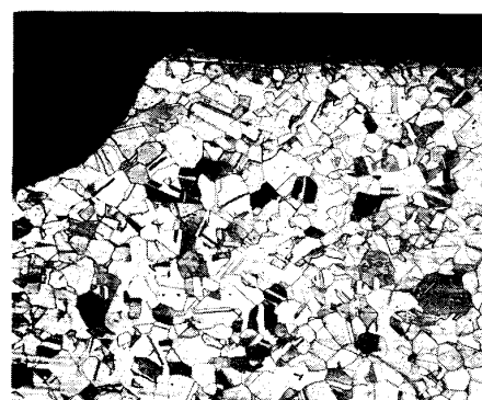
Photo 1. Oxalic acid etch test* result at heat affected zone of stainless steel (plate A) (* JIS G 0571)
