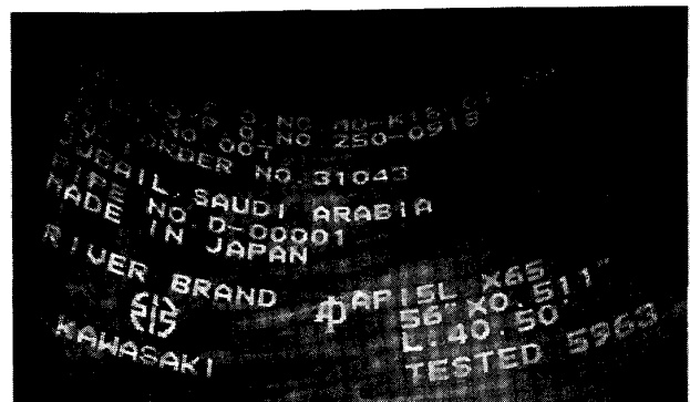
Photo.1 Automatic UOE marking
