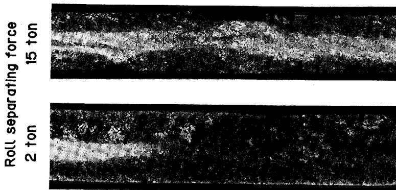
Photo 2 Effect of roll separating force on surface crack and segregation in twin-rolled cast sheets.
