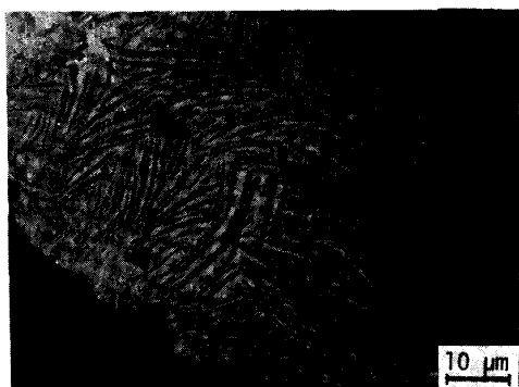
Fig.7 ε phase in Fe-4C-3Si
