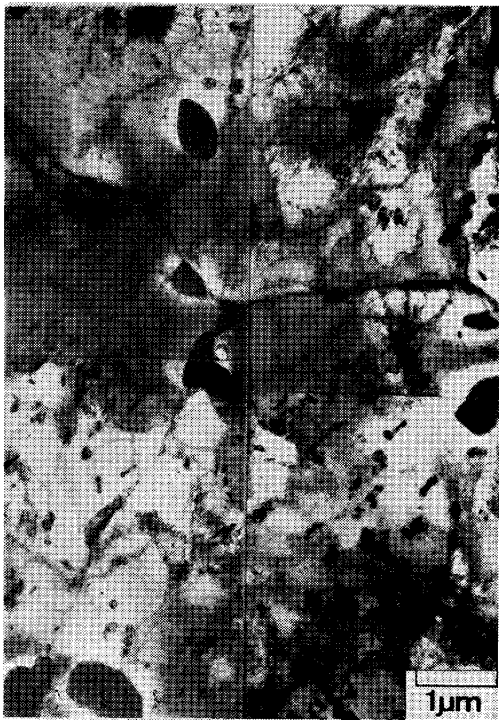
Photo. 6. Transmission electron micrograph of specimen crept at 600°C for 9000h ( \sigma : 10kgf/mm 2 ).
