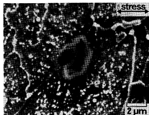
Photo. 3. Scanning electron micrograph of cracks associated with non-metallic inclusions found in specimen crept for 9000 h at 600°C ( \sigma : 10kgf/mm 2 ).
