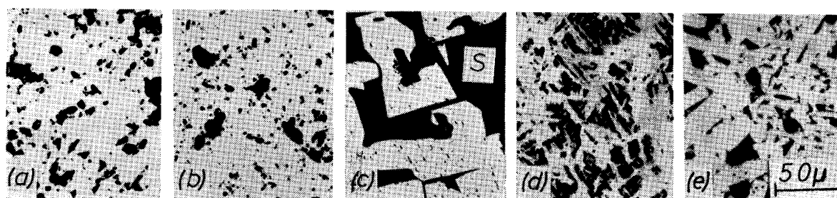
(a) Fine hematite (H-2) (b) Fine calcium ferrite (CF-5) (c) 2ndary hematite (H-10) (d) Needle type calcium ferrite (CF-8) (e) Prismatic calcium ferrite (CF-24)
