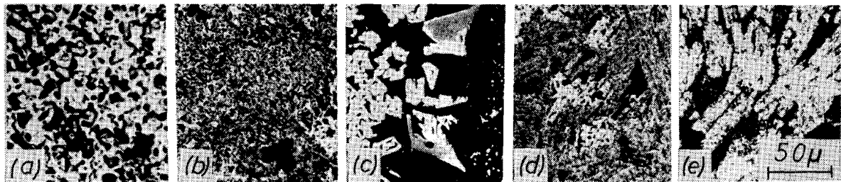
(a) Fine hematite (H-2) (b) Fine calcium ferrite (CF-5) (c) 2ndary hematite (H-10) (d) Needle type calcium ferrite (CF-8) (e) Prismatic calcium ferrite (CF-24)
