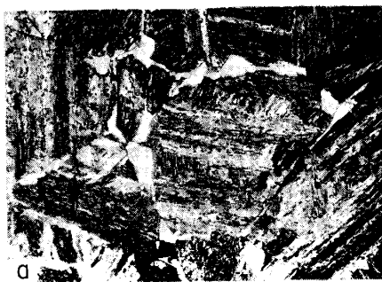
Photo. 1 Transformed at 680°C for 30 sec. (a) Not rolled, (b) 50% rolled.
