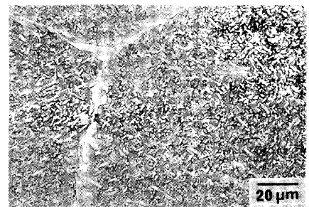
Photo. 2 Microstructures (Steel A, 1350°C W.Q. + 950°C \times 10 min).
