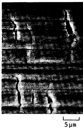
Photo. 1 Scanning electron micrograph of white streak
