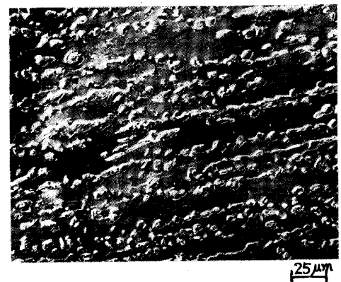
Photo.1 Microstructure of specimen hot rolled at 1100°C-70%R.D and held at 1100°C for 120 sec
