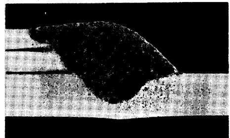
Fig.3 Macro section of weld
