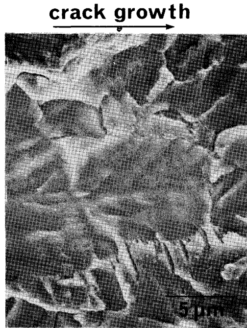
Photo. 4. Pearlite cracking revealed on the fracture surface due to hydrogen embrittlement of LT-specimen of steel B in as-rolled condition.
