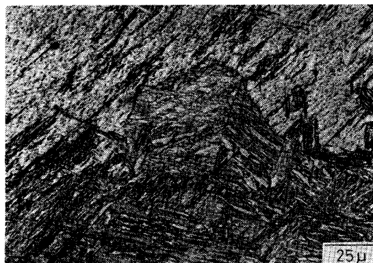
Photo. 8. Annealing twin in a small recrystallized austenite grain. Observation was made on the specimen reheated at 1250°C for 1 h, rolled 50% in 1 pass at 1050°C and quenched into water.
