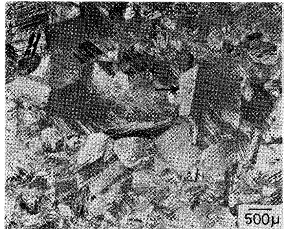
Photo. 1. Banded structure (see arrow) in the specimen simply reheated at 1250^\circ\text{C} for 1 h and quenched into water.
