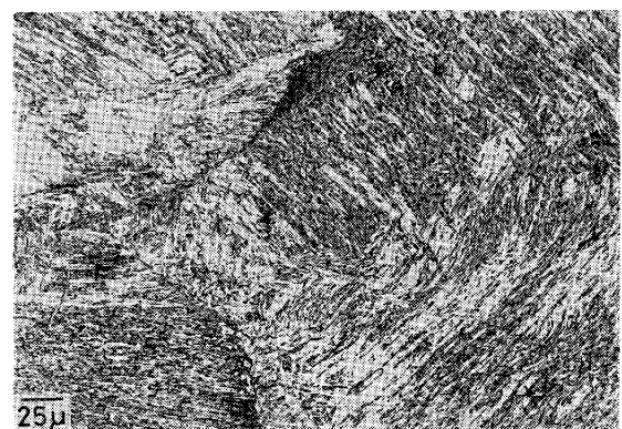
Photo. 6. Inhomogeneous deformation near austenite grain boundaries.
