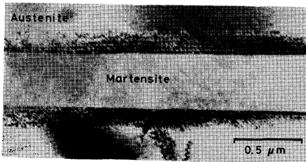
Photo. 8. Dislocations lying at the \gamma/\alpha' interface. Direction of dislocation lines coincides with the intersection of transformation twin plane with the habit plane 7) . (Fe-31Ni-0.3)
