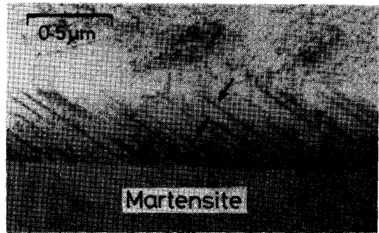
Photo. 15. Dislocations at martensite-parent phase interface, involved in the reaction of the dissociation to produce lattice dislocations in parent phase 4) . (Cu-37.65at%Zn)
