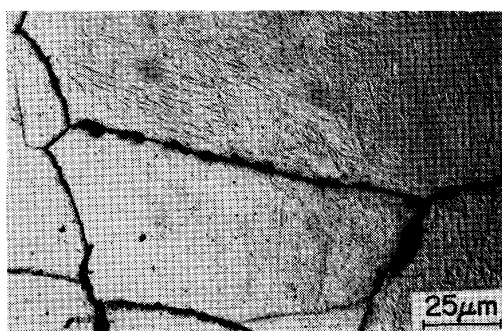
Photo. 2. Optical micrograph taken from the deformed specimen showing small pearlite nodules nucleated on the austenite grain boundaries in the early stage of transformation. Specimen was held for 10 min at 715°C after 30% rolling. Pictures were taken from the section (a) shown in Fig. 3.
