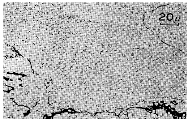
Photo. 1. Optical micrograph showing sulfide precipitates at 1/5 depth under the surface of hot rolled sheet of 3%Si-Fe added 0.17%Cu.
